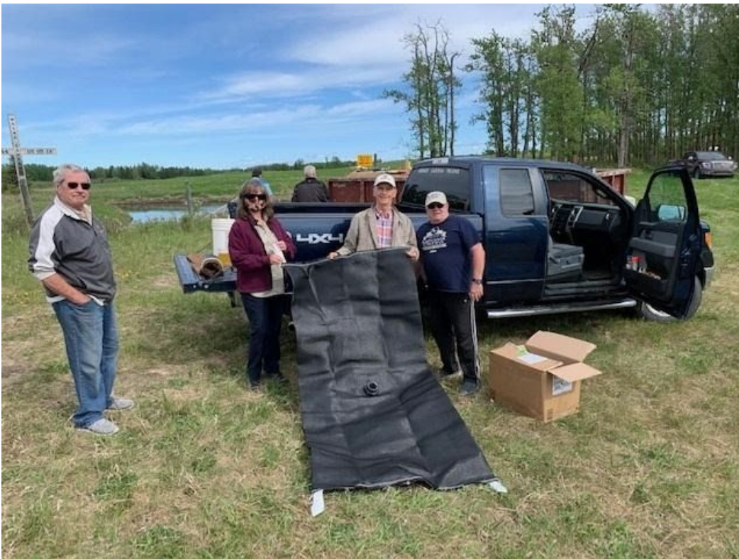
A test size Geotube filter before starting the test note the flanged inlet on top
