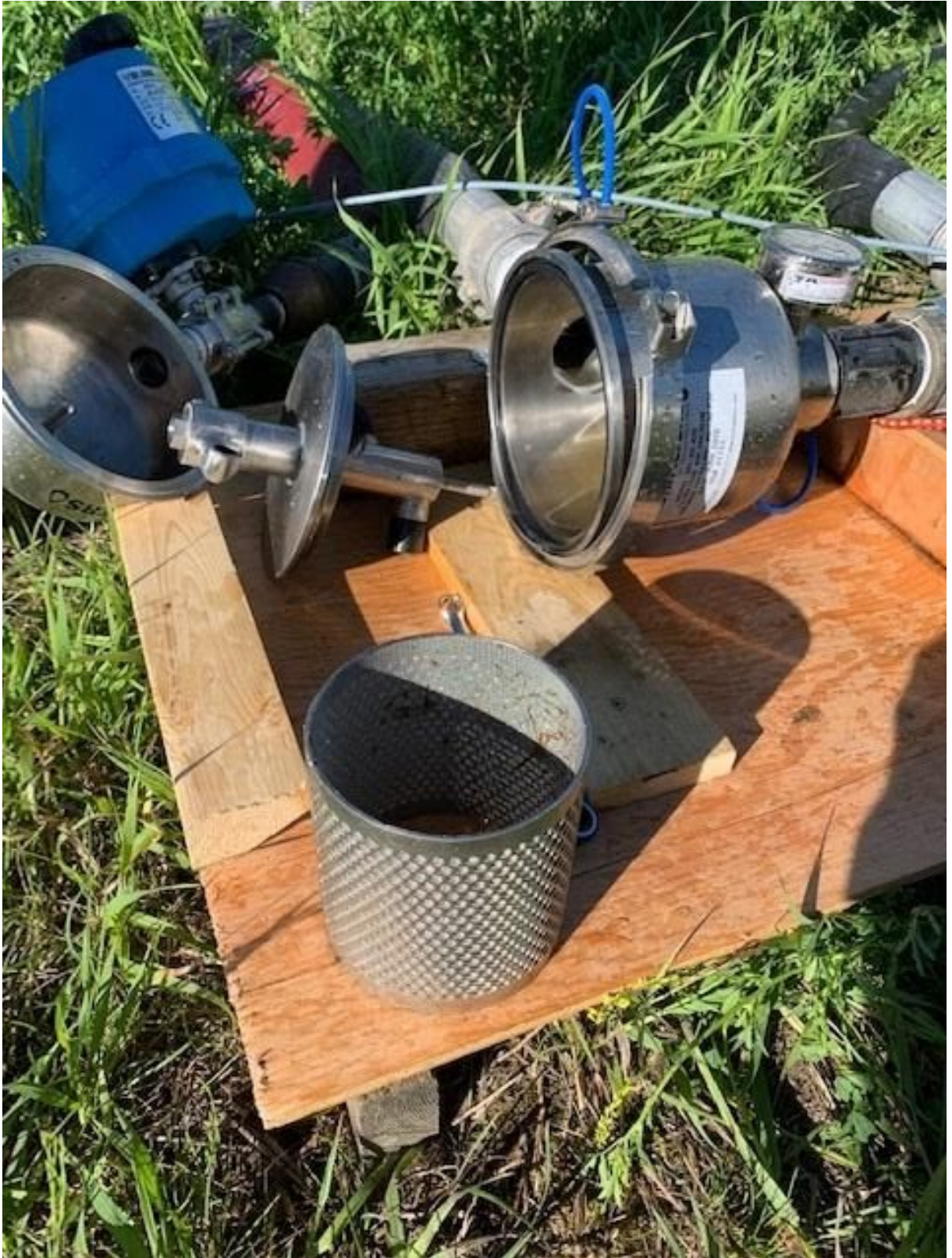
The disassembled filter showing the Forsta Filter cartridge beside the case with the backwash mechanism to the left
