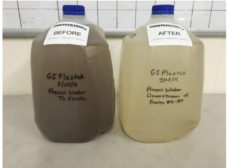
1 Gallon Samples BEFORE & AFTER the B4-180 Self-Cleaning Filter
