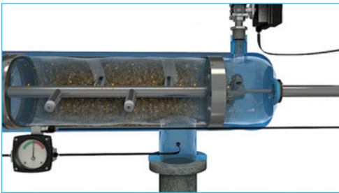
Suction nozzles vacuum particles from a dirty screen during the backwash cycle without interrupting the continuous flow of water through the filter.
